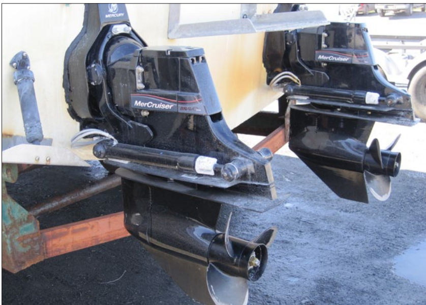
Tabs (far left, midway) outboard of twin outdrives help the boat maintain proper trim.
